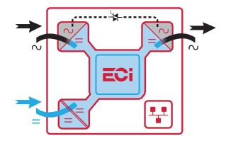
The ECI technology eliminates all single points of failure with full scalability; up to 32 modules in parallel and high efficiency of up to 96% in AC to AC conversion, and above 94.5% in DC/AC conversion, hence reducing operating costs. We can build the systems up to 2.7 MVA.
